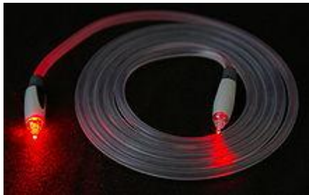
A TOSLINK optical fiber cable with a clear jacket. These plastic-fiber cables are used mainly for digital audio connections between devices.
